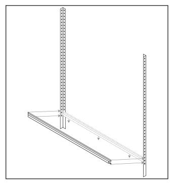
Figure 2. Attaching long shelf support.
